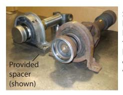
Step 4: Do not forget to include the rectangle spacer block... This is necessary to provide the same bearing height that was used on the OEM design Ford Trucks... the photo has the spacer under the service kit to show how it will provide the same center line height as the original. It must be included when you're ready to weld, balance and install the assembly.
