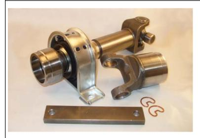
The OEM Ford rear drive shafts have a Non-replaceable center support bearing. With the Rockford Kit you are able to cut the Original assemblies apart at the friction weld and replace the Slip Yoke, Splined Stub and Center Support Bearing... avoiding the addtional cost required to build an entirely new assembly.
