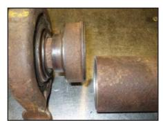
Step 1: Cut the original tube right behind the friction weld on the stub of the center support bearing and then again behind the friction weld of the splined stub and original tubing.
