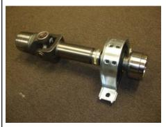
Step 3: The proper way to assemble the Rockford kit is illustrated with the photo shown. The midship stub shaft is pressed into the front OEM tube and welded in place. The weld yoke is pressed into the rear OEM tube and welded.
