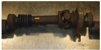
The OEM Ford rear driveshafts have a non-replaceable center support bearing. With the Rockford Kit you are able to cut the Original assemblies apart at the friction weld and replace the Slip Yoke, Splined Stub and Center Support Bearing..
